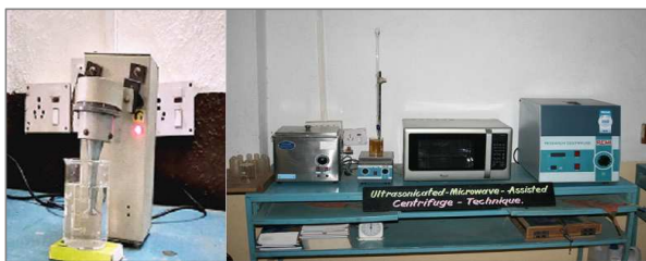
Fig. 1: Disc type ultrasonicated microwave assisted centrifuge technique
