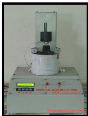
Fig.1. Automatic Chemical Bath Unit (A-CBD unit)
